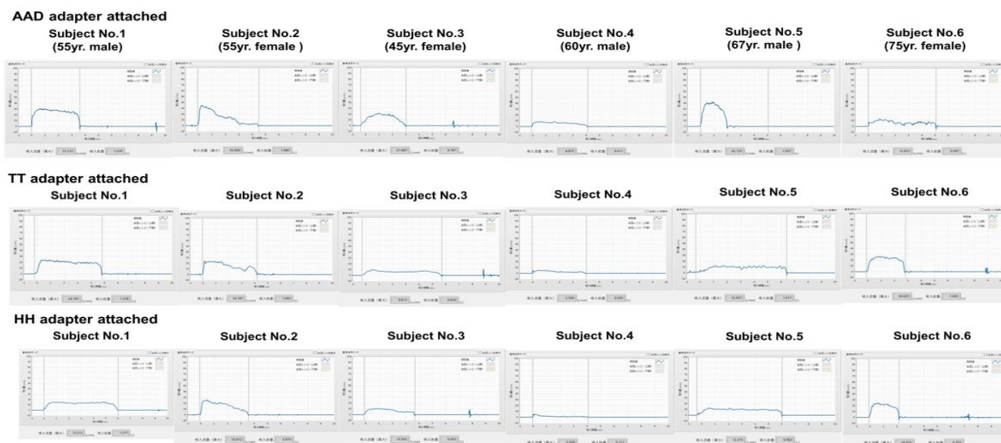
Figure 5: Comparison of inhalation patterns of individual subjects under the instruction “Inhale as if sucking juice through a straw”.
